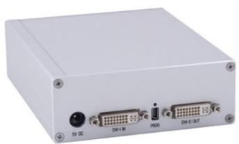
The new **TLS Converter & Scaler AD/D** converts analogue input signals into digital signals and allows for connecting DVI devices such as projectors, TFTs and LCDs to analogue sources such as the VGA output of a graphics card.
