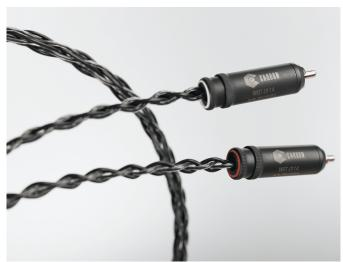
The Carbon in the names refers to an electrostatically dissipative carbon polymer used between the Teflon dielectric and VariStand 19.5 AWG conductors. The company says the manufacturing technology reduces mechanically induced electrical noise in the cable and improves the uniformity of the voltage gradient within the insulating dielectric.
