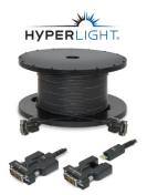
The cables are HDCP 1.4 compliant and support signals with aggregate data rates up to 4.95Gbps. Such features enable HyperLight cables to support any single-link DVI resolution with cable lengths up to 328m. Construction is in a hybrid design of four POF (Polyfluorinated Optical Fiber) and 6 copper wires, allowing for a rugged and flexible cable with a minimum bend radius of only 2mm.
