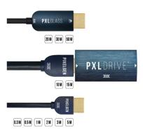
Described by the company as the first fibre-based long reach 4K interconnect solution with THX certification, PXLGLASS delivers 100% uncompressed 4K signals and the full HDMI feature set. To do so it uses a unique copper/fibre hybrid cable implementation, with optical fibres carrying high-speed TMDS signals while copper-based wires carry critical low-speed communication signals such as HDCP 2.2 and CEC 2.0.
