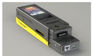
The built-in HDMI pattern generator supports both CEA and DMT resolutions up to 4K/28Hz, making it compatible with virtually every AV source and display device available. A 3.5-inch touchscreen displays basic performance diagnostics for fast analysis of connectivity signals, including go/no-go indication, cable length, pixel clock and Tx/Rx overall performance.
