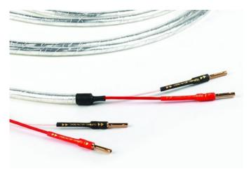
A refinement on recent Chord Company developments, Clearway Cable features 2 contra-wound high-density foil shields allowing for a shielding level effective to high frequencies. Meanwhile a clear protective PVC jacket reduces mechanically induced noise.
