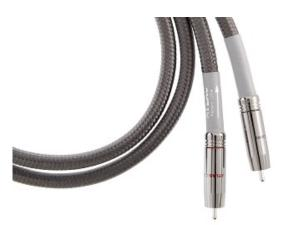
The cable features a conductor made out of a single solid core surrounded by 64 interwoven strands of Ohno Continuous Cast (OCC) grain-free copper. In turn the fluorinated ethylene propylene (FEP) is extruded around the bare OCC copper conductors in a thermally stable manner, a process offering greater manufacturing consistency and wider bandwidth.
