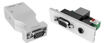
Audio passes through the transmitter, but VGA is sent to the receiver which plugs directly into the projector - via twisted pair cable up to 60 metres long. A power-over-ethernet system means only one mains power adaptor is required to power both the transmitter and receiver – and this can be used at either end.
