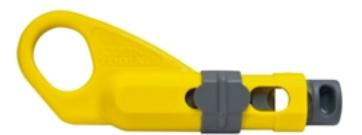
It provides 2-level (outer jacket and dielectric [7.9mm and 6.4mm]) stripping in 1 step, as the sliding depth gauging removes guesswork out of repeatable cable end preparation. It also prevents installers from using their fingers as a backstop on sharp wire tips.
