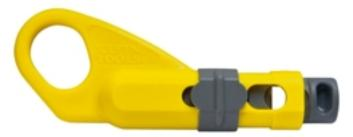
It provides 2-level (outer jacket and dielectric [7.9mm and 6.4mm]) stripping in 1 step, as the sliding depth gauging removes guesswork out of repeatable cable end preparation. It also prevents installers from using their fingers as a backstop on sharp wire tips.
