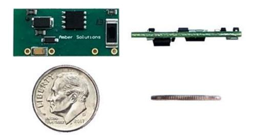
The AC/DC Enabler is a patented, UL-certified and globally compatible 30 x 15 x 8mm solid-state digital power management and control system. Combined with the patented Amber AC Switch, the two foundational technologies represent a "breakthrough" in the software management of electricity through solid-state architecture. Amber says it has already integrated the technology into fully demonstrable solid-state products, such as a smart programmable retrofit circuit breaker.
