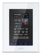
The KX3 combines an in-wall touchscreen and a control processor into a customisable and powerful easy to use unit. It is complete with proximity sensor and room status LEDs, while installation options include wired 10/100 Base-T ethernet and wireless ethernet capabilities for viewing video from network security cameras and remote programming updates.
