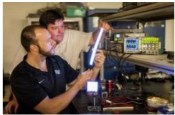
Called FIPEL (Field-Induced Polymer Electrolumeniscent), the technology consists of 3 layers of moldable light-emitting polymer (aka plastic) blended with a small amount of glowing nanomaterials. Once an electric current is applied the system produces a bright white light without the harsh, bluish tint LEDs tend to have
