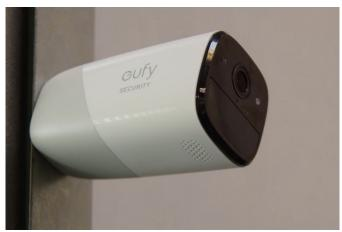
The EverCam promises to run wire-free on a battery (a 13400mAh lithium-ion number from Anker) allowing up to 1 year of use on a single charge. Further boosting battery life is a low-power standby mode ensuring the camera only wakes up and starts recording whenever motion is detected, as well as connectivity with an indoor base station using a low-frequency wireless protocol. In turn the base station connects to the internet and users' PCs and smartphones via wifi.
