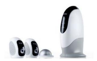
The wireless cameras transmit up to 100m to the nearest gateway. They mount on custom sticks via magnetic mounts, and easily relocate as needed. The cameras shoot video in flv at up to VGA resolution, and use FrameMesh wireless video encryption. Vuezone says battery life is up to one year under normal usage.
