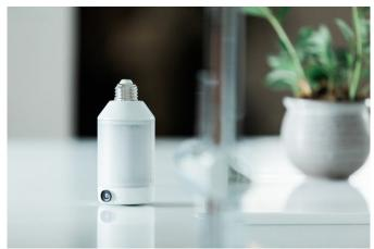
The LightCam is a combination of security camera and smart light bulb. It should fit in any standard light socket, with a 1080p camera complete with IR sensors pushing images (as triggered by motion sensors) to companion smartphone app. Built-in storage records around 7 days of footage, and users can add more storage space through backups to smartphone, PC or cloud storage. Built-in speakers and microphone provide 2-way communications.
