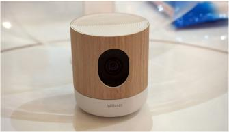
The camera portion features a 135-degree wide-angle zoom and "clear" night vision, allowing it to detect both general motion and the presence of people. Meanwhile the microphones detect sound and specifically recognise crying, allowing use as a baby monitor.
