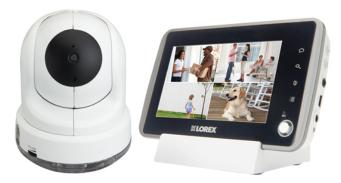
Setup also requires no PC, since an included Wifi Cradle takes care of connections with home wireless networks. Once the Cradle connects to a wifi network, customers just need to dock the monitor to view video either remotely or locally.
