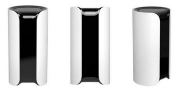
The device is 15cm tall and 7cm wide and features motion, temperature, humidity and air quality sensors together with an HD camera (with night vision and wide angle lens), microphone and siren. Once placed on a shelf or plugged into a wall the Canary records and uploads data to a cloud-based service (available in either free or paid subscription flavours) users can access via web browser or smartphone app.
