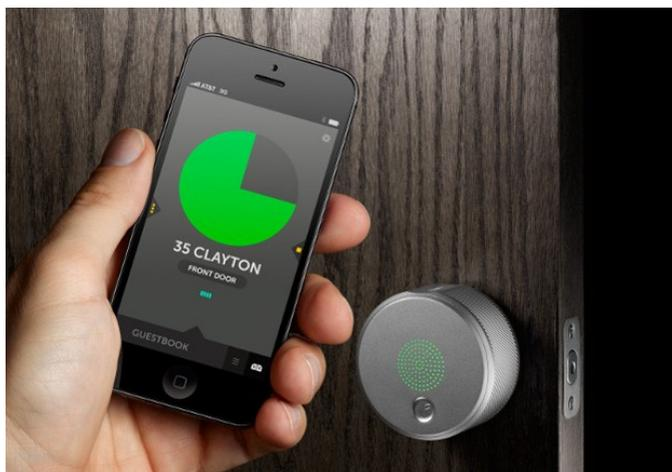
Making the lock module rather interesting is not the striking Yves Behar industrial design (although it does remind us of the Nest thermostat) but its security features. It uses BLE and a paired smartphone or tablet instead of wifi to connect briefly with the August online service. Once the module syncs with the service it assigns an algorithmically generated key to the paired mobile device, thus avoiding the risk of hacking internet connections involve.
