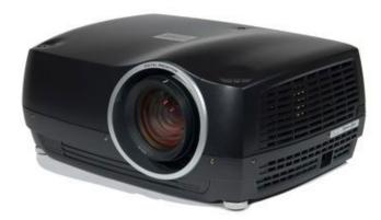
The dVision 31-1080p 3D uses single chip DLP technology to produce up to 2900 lumens of brightness and contrast rations of up to 7500:1.
