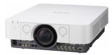
The technology uses a blue laser light source to excite a phosphorous material into generating white light. The 3LCD optical system splits the white light into RGB, producing 4000 lumens of light at WUXGA (1920x1200) resolution and what Sony claims is "bright and vivid color reproduction."
