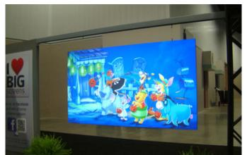
To meet modern demands for wider, flatter screens, the dnp Supernova Blade is only 3mm thick and available in 100", 110" and 120" displays (in 16: 9 aspect ratio). Yet it contains the performance characteristics typical of a Supernova Screen.
