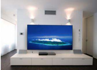
The Black Diamond Motorised uses Black Diamond ambient light rejection screen technology, a material SI claims reduces light scatter by over 75%. With 1 motor, 4 custom helixes and a spool of slender aircraft cable, Black Diamond Motorised lowers a thin wing containing the rolled screen downward from a recessed ceiling-mounted cassette.
