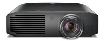
Upgrades in the PT-AT6000E include a new 220W "Red Rich" lamp, boosting brightness to 2400 lumens and contrast to 500000:1 (up from 300000 in the PT-AT5000E).
