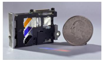
Current LC projectors generate light from unpolarised light sources (such as LEDs) before passing it through a filter. However filters "waste" around 50% of originally generated light, turning it into heat... the reason projectors need (generally noisy) cooling fans.
