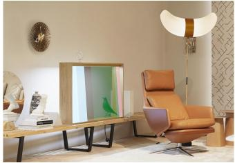
The transparent OLED display consists of a wooden frame holding what appears to be a pane of glass. However, once the device is turned on, it transforms into an OLED display. Designed by Scandinavian based designer Daniel Rybakken and Panasonic Design Kyoto, the display features materials such as wood, metal and glass, with the wooden frame hiding all electronic components and housing a lighting element.
