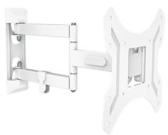
Both mounts are built out of 2.5mm cold-rolled steel, allowing for increased tensile strength and finer surface tolerance. The VFM-WA2X2v2 takes VESA sizes up to 200x200, and the WA4X4v2 takes sizes up to 400x400. Both have a 402mm reach, -2-12° tilt and 90° swivel adjustment. To help with installations, the mounts have 6° of rotation in case the wall bracket is not fixed plumb.
