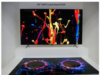
The concept for the technology is based on the wafer-thin nature of OLED panels. A pair of tiny speaker drivers can deliver audio signals to the panel, causing it to vibrate in order to produce sound. The two companies claim the result is more immersive than traditional TV speakers, since the sound comes directly from the screen, as opposed to from below or beside it.
