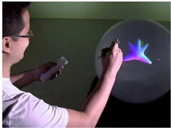
Described as the first "3D perspective-corrected interactive spherical scalable display," Spheree was revealed at the SIGGRAPH 2014 conference. In another mouthful from the team, it "arranges multiple blended and calibrated mini-projectors to transform a translucent globe into a high-resolution perspective-corrected 3D interactive display."
