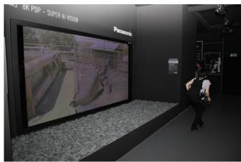
A Panasonic and NHK co-development, the Super Hi-Vision TV carries a self-illuminating plasma panel and handles resolutions of up to 7680x4320. Positioned down a narrow hallway, it was also admittedly difficult to photograph properly.
