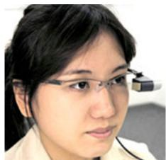
Brother Industries prototypes a wearable display that fits like a pair of eyeglasses and bounces light into the retina to create the sensation of viewing a floating image.
