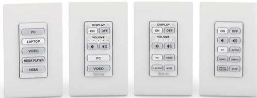
Network Button Panels connect to a control processor using standard ethernet. The customisable control panels work in conjunction with an IP Link Pro control processor HC 400 series system to perform a wide range of AV system functions, including display on/off, input switching, volume control and more. The buttons are easily customisable using an online Custom Button Builder Application, while PoE allows for both power and communications over a single ethernet cable.
