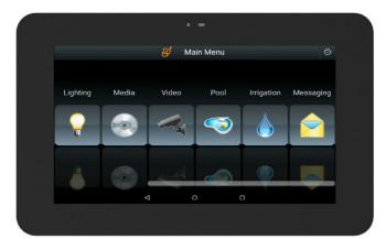
The gXP12 has an 11.6-inch 16:9 display offering 1920 x 1080 resolution together with a 5MP camera. Designed for ELAN Intercom, the touchpanel provides high-fidelity audio for clear conversations and notification chimes, as well as a digital MEMS microphone with echo and noise cancellation.
