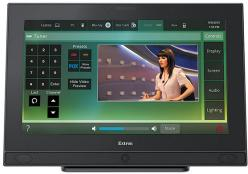
The TLP Pro 1220TG features video preview inputs that support high resolution HDCP-compliant video from HDMI sources and Extron XTP devices, while the TLC Pro 521M features a secure and powerful built-in control processor and ethernet-controllable device support. All three touchpanels feature faster processing and more memory.
