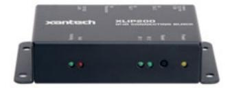
The XtraNet XLIP200 is a basic IR input and output device. It supports native IR I/O over wired networks (to which it interfaces via an RJ-45 connector) and is configured as an input by default.
