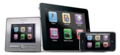
The 6 series handles key technologies including Apple TV, blu-ray, iDevices, DAB/DAB+ streaming and internet radio-- together with lighting, heating, windows/blinds and CCTV control integration (including KNX devices).
