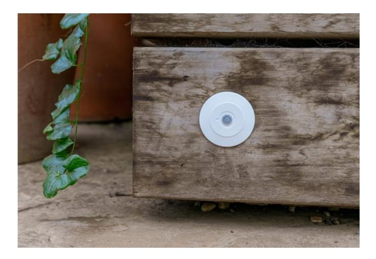
Ideal for use bout inside or outside, the sensor is rated as both dust tight and protected against immersion in water for 30 minutes at depths of up to 1000m. It is powered by 5-35V DC, and provides fully volt-free output. According to the company, it covers a 5 x 5m detection area from a height of 2.5m. Installers can integrate it with a number of control platforms, including Loxone, Crestron, Control4, Lutron and Rako.
