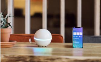
Founded by Emile Nijssen and Stefan Witkamp in 2014, Athom created Homey, a product combining all wireless and smart devices into a single system. The small spherical device carries a total of 7 radios for wifi, Bluetooth LE, Z-Wave Plus, NFC, 433MHz, 868MHz and ZigBee connectivity, and also includes an ethernet port.
