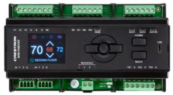
The DIN-THSTAT provides 3-stage heating and cooling, support for x3 independent remote sensor inputs (through the Crestron CHV-RTS, CHV-RTHS, or CHV-RSS temperature sensors), full colour LCD display for easy setup and diagnostics, and flexible Cresnet communications. It installs in an equipment cabinet or a wall, and the cabinet can be flush or surface mounted.
