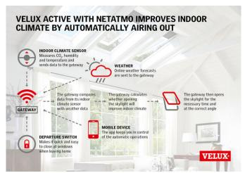
First announced back at CES 2017, the Velux Active skylights automatically adjust open/close levels, as well as motorised shades. The solution includes a wifi gateway and controls for Velux Integra roof windows and sunscreen products, plus an iOS/Android control app. As for sensors, the company offers weather gauges, rain gauges, wind gauges, security cameras and indoor air quality monitors, and the "with Netatmo" program allows integration into smart home systems.
