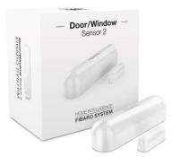
The Door/Window Sensor 2 connects to either the Fibaro Home Center ecosystem or a Z-Wave hub, and is accessible through companion app on smartphones, tablets or browser. It monitors the status of the door, window, gate or blinds it is connected to, and reports back any change in open/door status, helping avoid theft, break-ins or energy loss if a door is left unintentionally open.
