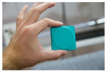
The Pop buttons feature 3 control gestures, and connect to devices via bridge device able to pair with an "unlimited" number of buttons. As for HomeKit, one simply needs to pair the bridge with the Apple Home app before configuring required scenes. The company adds Pop buttons are compatible with non-HomeKit devices, such as Sonos wireless music systems, Osram lighting, Hunter Douglas and Lutron blinds, and more via companion Pop app.
