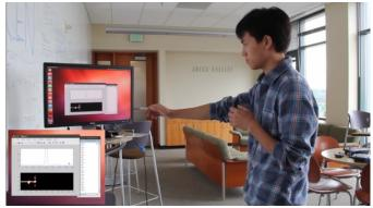
The technology measures the so-called "Doppler frequency shift" caused in wireless signal frequency by body movements. Such frequency changes are very small (several hertz compared to 5GHz wifi signals), yet UW says the technology identifies up to 9 different whole-body gestures through a clever algorithm measuring these slight shifts.
