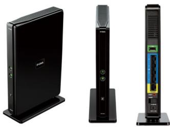
It uses the 5GHz band for "less interference and cleaner connection" and carries x4 ethernet ports and x1 USB port allowing the connection of external storage. It is IPv6 ready and backwards compatible with 802.11n wireless standards.
