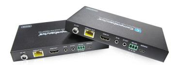
The kit converts HDMI signals to a standard HDBaseT signal before transmission over a single ethernet (Cat5e or higher) cable. It also supports bi-directional POC, eliminating the need to run additional power, and includes x2 IR receivers and x2 transmitters to allow for bidirectional infrared control of a connected HDMI source and display.
