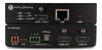
A successor to the Atlona AT-HD-M2C and AT-UHD-M2C-BAL, the ATR-HDR-M2C extracts, decodes and downmixes multi-channel PCM, Dolby and DTS audio from HDMI sources, and delivers stereo downmixed audio over HDMI, analog unbalanced audio and TOSLINK digital audio outputs. It also simultaneously pass through the HDMI input with no downmixing.
