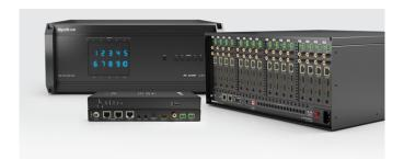
The H2X matrix switcher series is designed for large, high-end residential and commercial applications demanding multi-source video distribution of 4K HDR content, as well as multi-source audio matrix switching to multiple zone. A SmartEDID feature dynamically detects and reacts to display and source capabilities to output the highest possible resolution for each source, while the addition of the RX-70-4K-SCL HDBaseT scaling receiver adds 4K-2K scaling and frameless switching.
