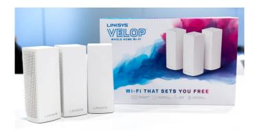
The Velop system uses a tri-band 802.11ac MU-MIMO mesh network, with one band dedicated to communication between routers to prevent some of the bottlenecks two-band systems suffer from. The routers also include two ethernet ports in case customers prefer cable connectivity. The mesh system is self-healing, and can handle up to 5 Velop units to ensure wifi coverage in even the largest of houses.
