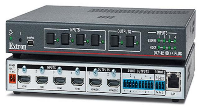
In order to maintain signal integrity and reliability, the switcher provides automatic cable equalisation on each input and independent output reclocking to reshape and restore video signal timing on both HDMI outputs. EDID Minder and Key minder ensure what Extron says is optimal system performance and compliance with HDCP-encrypted content.
